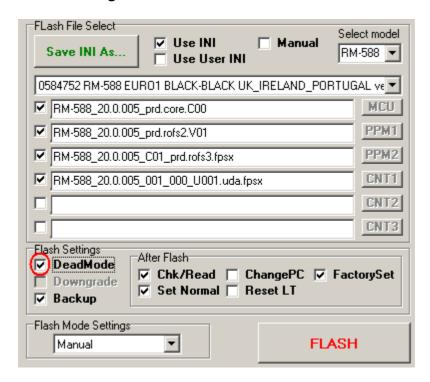
After that choose the firmware file and press the FLASH button, next connect the phone and finally shortly press the power button. If the flashing operation is successful - the phone will be set to the TEST mode and the program will wait for further user commands.
